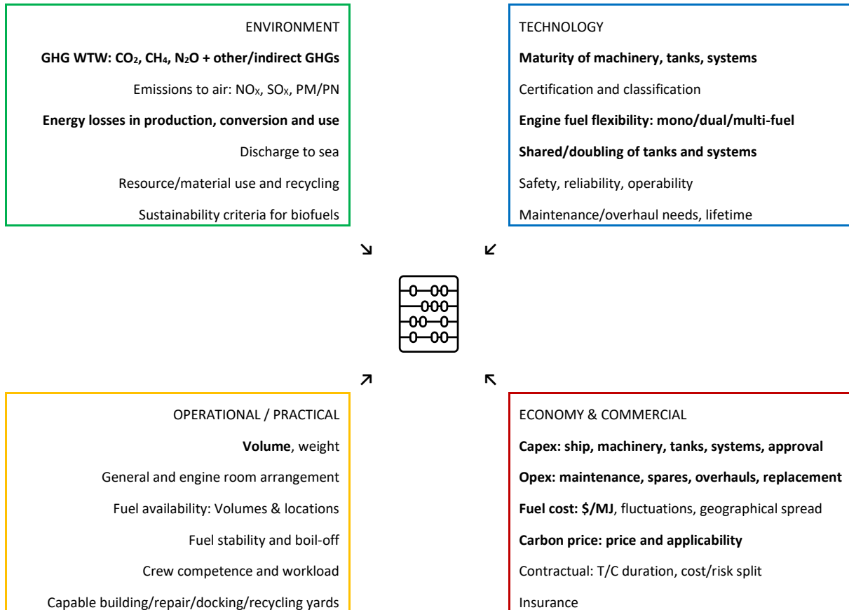
Figure 7: Evaluation criteria for alternative fuels [Gamlem, Smart Maritime Sea map to green shipping , 2023].
