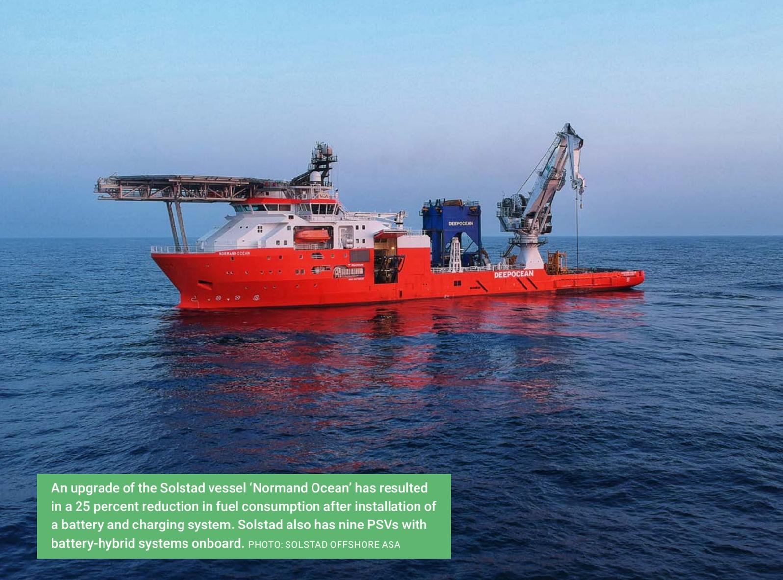
An upgrade of the Solstad vessel 'Normand Ocean' has resulted in a 25 percent reduction in fuel consumption after installation of a battery and charging system. Solstad also has nine PSVs with battery-hybrid systems onboard. PHOTO: SOLSTAD OFFSHORE ASA
